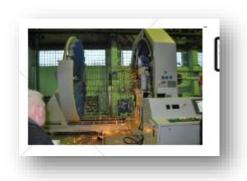
Welding cage machine for producing cages for pipes and manhole rings; producer mbk Maschinenbau GmbH (Germany), type BSM 450 - 33-300/24 LD 3000, construction year 2009,
