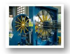
Welding cage machine for producing cages for pipes and manhole rings; producer mbk Maschinenbau GmbH (Germany), type BSM LB - 22-190/12 LD 3000, construction year 2008, new, was not in use
