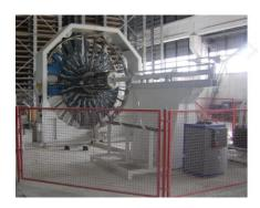
Welding cage machine for producing cages for pipes and manhole rings; producer mbk Maschinenbau GmbH (Germany), type BSM 450 - 33-300/24 LD 3000, construction year 2008
