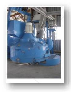
Concrete – mixing equipment with line the of bucket concrete supply (SCHLOSSER-PFEIFFER, Germany), construction year 2008
