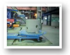
Machine for drilling holes in the manhole rings with nozzles KRB 650 (Germany), construction year 2009
